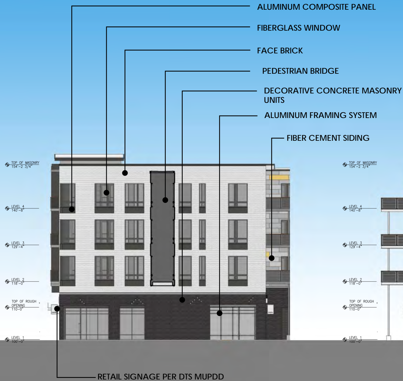
1 - BUILDING A AT BRIDGE - NORTH ELEVATION
