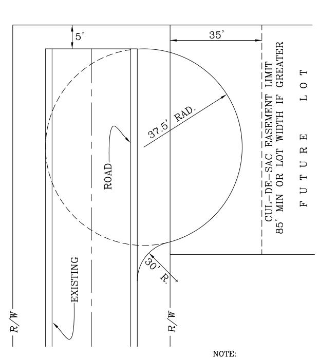
NOTE: TEMPORARY CUL-DE-SAC SHALL HAVE A MINIMUM DIAMETER OF 75' AND CONSIST OF A 6" STONE BASE WITH 3" OF ASPAHLT.
