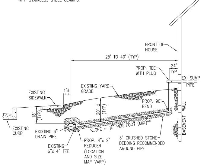
\*\* - THE SLOPE MUST BE AT A MIN. OF ¼" PER FT., REGARDLESS OF THE SIZE OR TYPE OF PIPE USED, OR THE LOCATION OF THE REDUCER.
