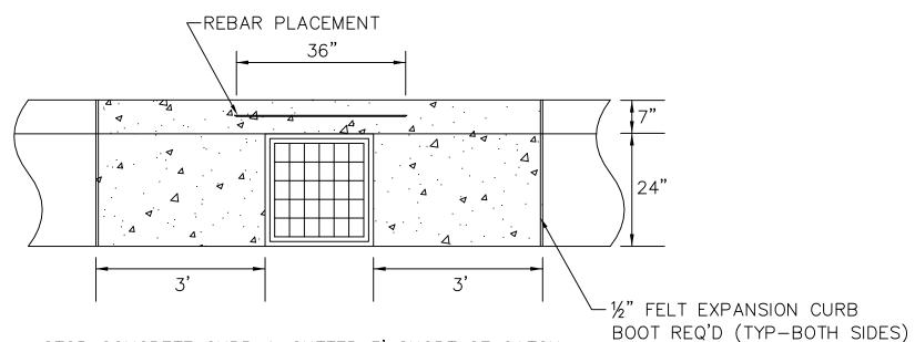
STOP CONCRETE CURB & GUTTER 3' SHORT OF CATCH BASIN CASTING, SET CASTING TO BINDER COURSE GRADE AND INSTALL TEMPORARY ASPHALT CURB & GUTTER.
