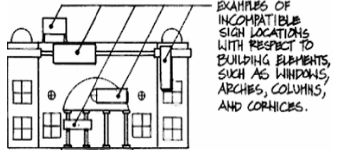
INAPPROPRIATE SIGN LOCATIONS
