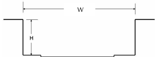
OPTIMAL STREET ENCLOSURE Building Height (H) = 1/3 Street Width (W)
