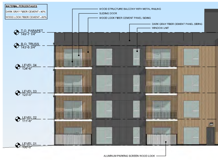
6 NORTH BLDG. - SOUTH ELEVATION 1/8" = 1'-0"
