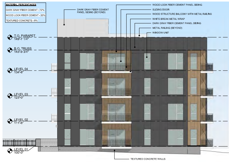
4 NORTH BLDG. - SOUTH ELEVATION 1/8" = 1'-0"
