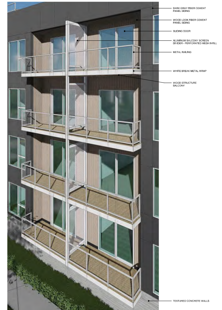
1 BALCONY SCREEN DIVIDER - PERSPECTIVE - NORTH BUILDING 1/2" = 1'-0"
