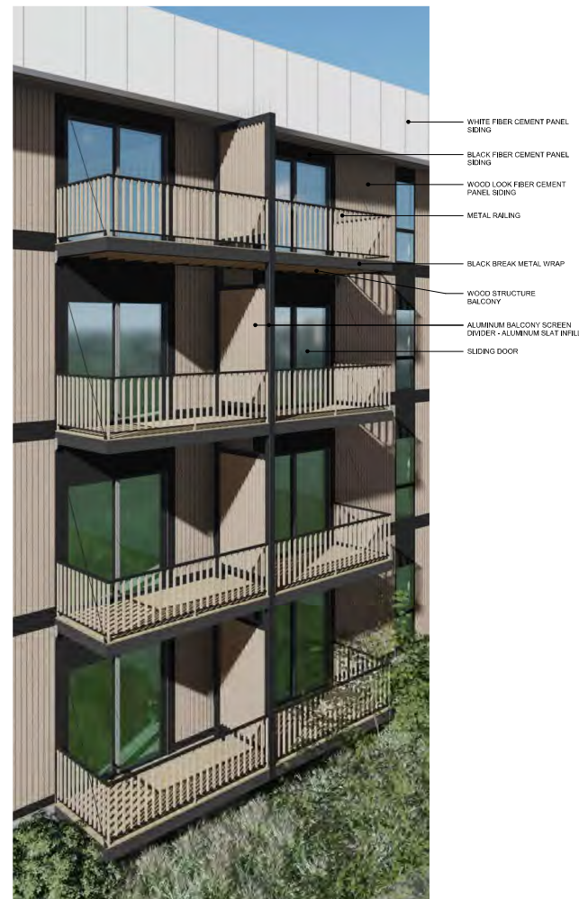
4 BALCONY SCREEN DIVIDER - PERSPECTIVE - SOUTH BUILDING 1/2" = 1'-0"
