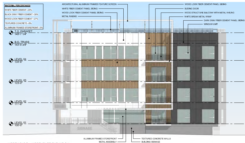
2 NORTH BLDG. - NORTHEAST ELEVATION 1/8" = 1'-0"
