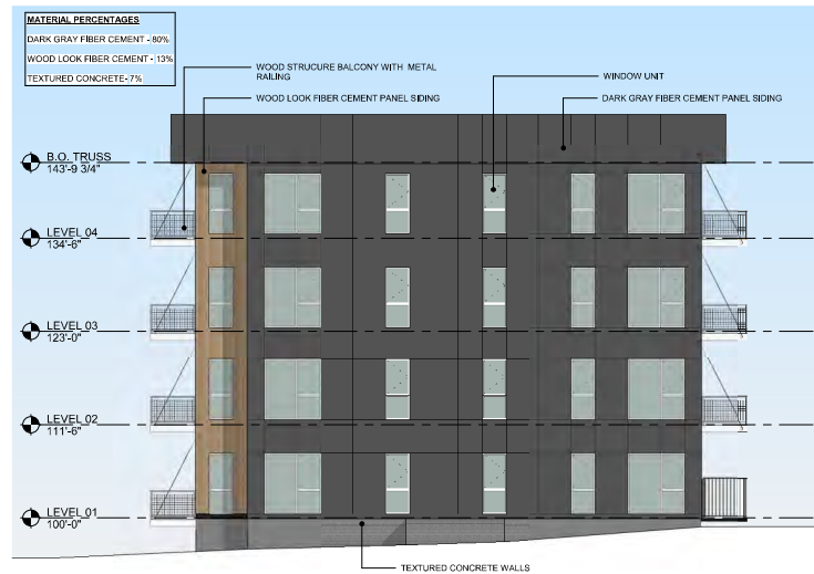
7 NORTH BLDG. - WEST ELEVATION 1/8" = 1'-0"
