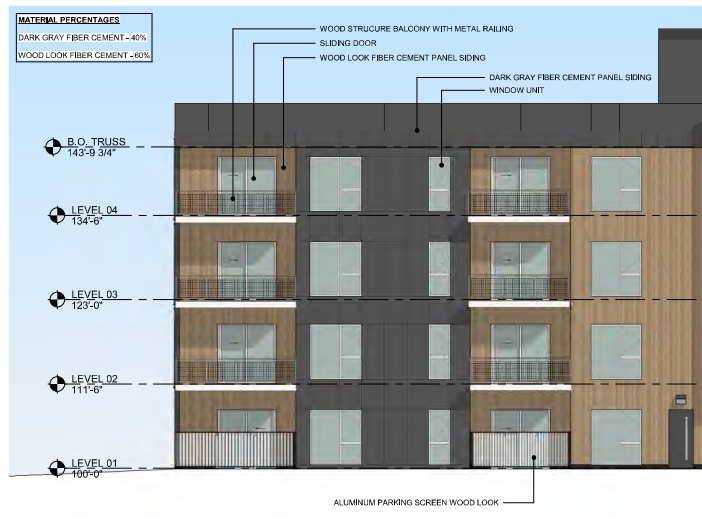
6 NORTH BLDG. - SOUTH ELEVATION 1/8" = 1'-0"
