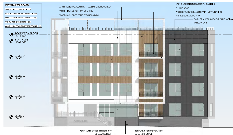
2 NORTH BLDG. - NORTHEAST ELEVATION 1/8" = 1'-0"
