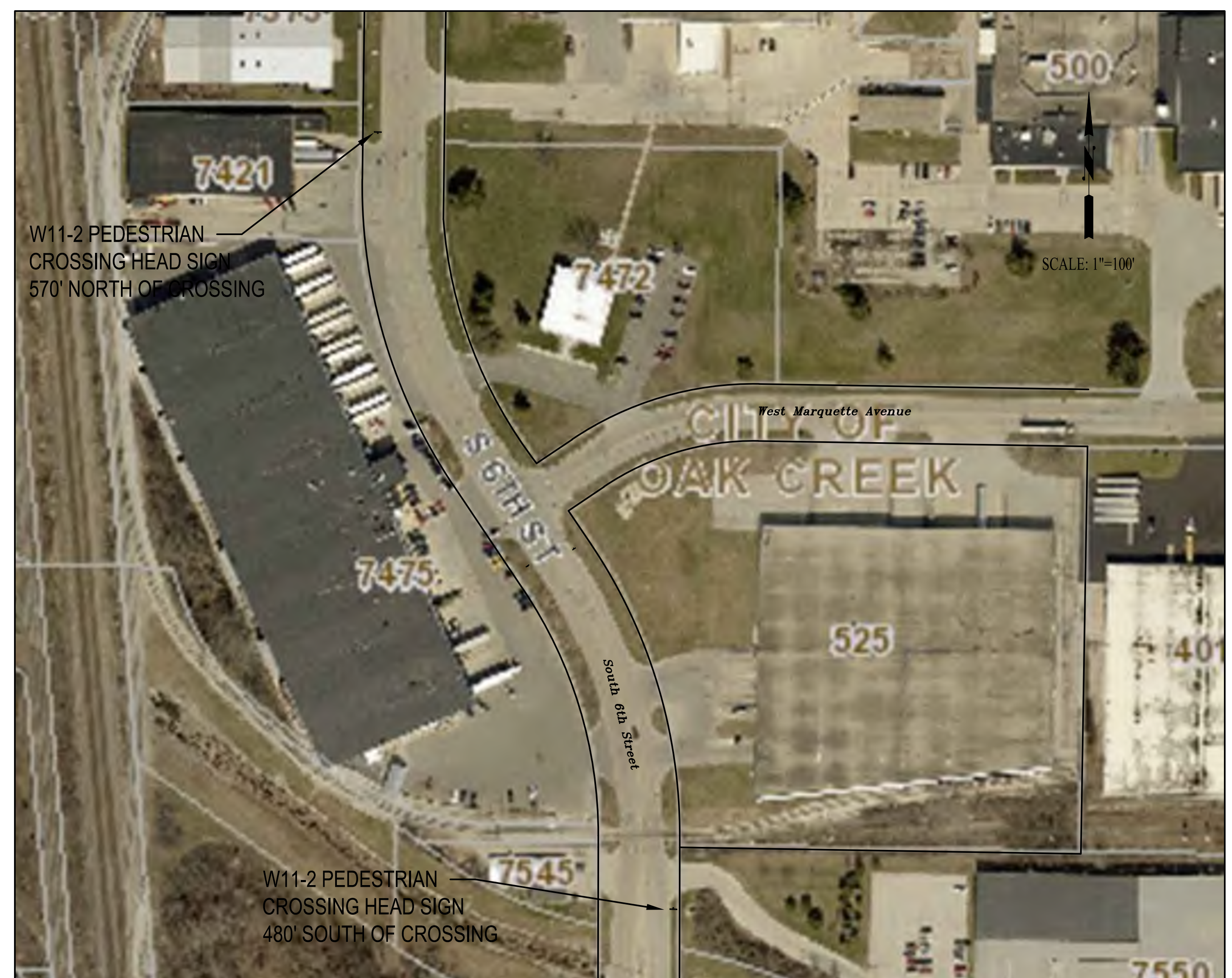
PEDESTRIAN CROSSING AHEAD SIGN DETAIL
