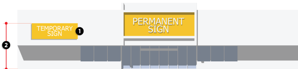
Figure 6.10: Wall Mounted Banner Sign Standards
