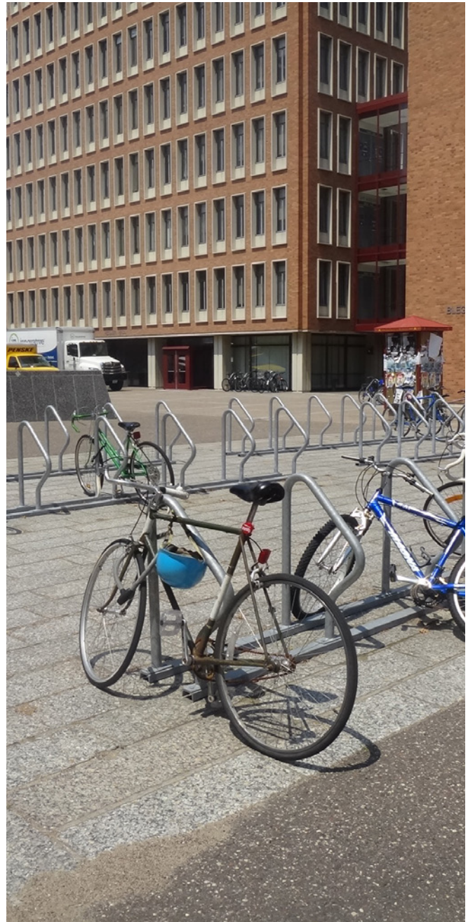
Arrangement of a bike parking area with a central aisle for circulation.
