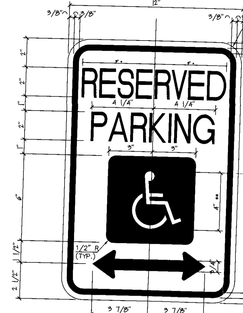
RESERVED PARKING SIGN Legend and Border: GREEN WHITE Symbol and BLUE Background Background: WHITE Reduce Spacing 50% See Symbol 'E' For Symbol Proportions ACCESSIBLE PARKING SIGN 3" = 1'-0"
