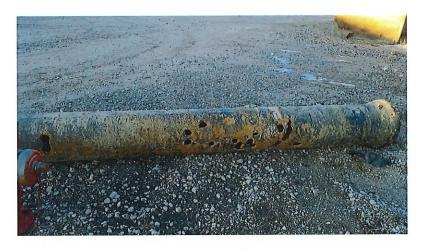
Given the physical condition of the pipe, and the length of time customers were without water service, relaying this water main is warranted. Approving this agreement will fast track the design of a new 12" PVC water main in Puetz Road between STH 32 and the railroad tracks.
